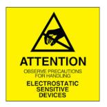
Warning: The device mounted on the PCB is an OEM module designed for system integration only, not for general uses. Do not touch the PCB by hand. The electrical static can kill the chips even without a power plug-in, and unpleasant electrical shock may also be felt. For laboratory use, please buy a protected Turnkey system.
